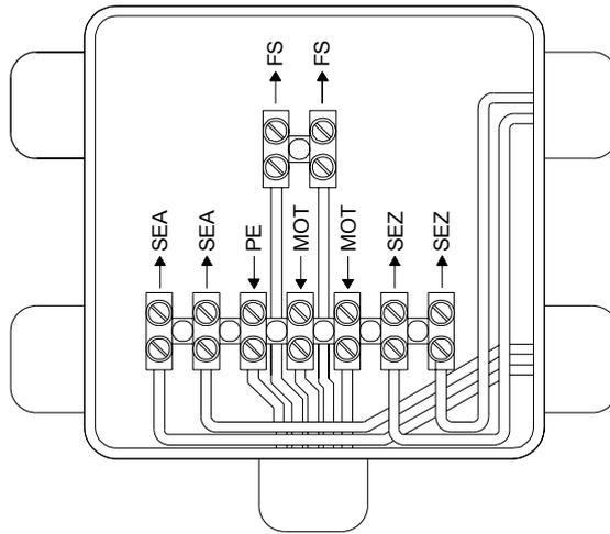
The controller MO 90 should be placed as near to the gate as possible (Best position is directly next to the controller of the gate opener). The control box should be mounted with the entrance for wiring at the bottom. The leads should have a cross section of at least 1.5mm<sup>2</sup>. The optimal installation would be a mutual installation of both controllers in one large controller housing.
