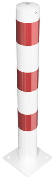
Barrier posts, steel tube  $\varnothing$  102 x 2,9 mm, stationary, to be fixed by plugs, hot-dip galvanized and white coated with three red reflecting stripes
