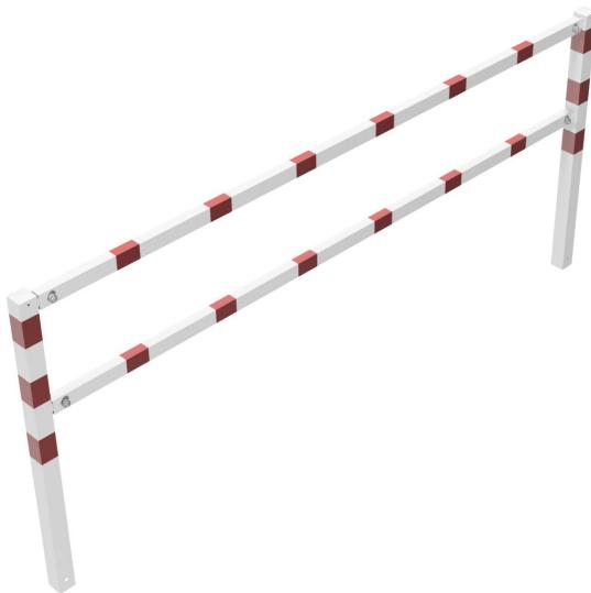
Stationary access barriers for bolting on site with top and quarter-bent bar, hot-dip galvanized and white coated with red reflecting stripes, total width: 3000 mm
